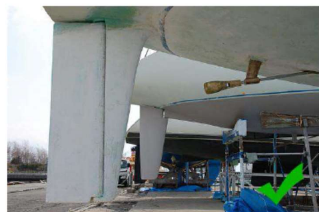
Skeg clearly visible as is propeller
